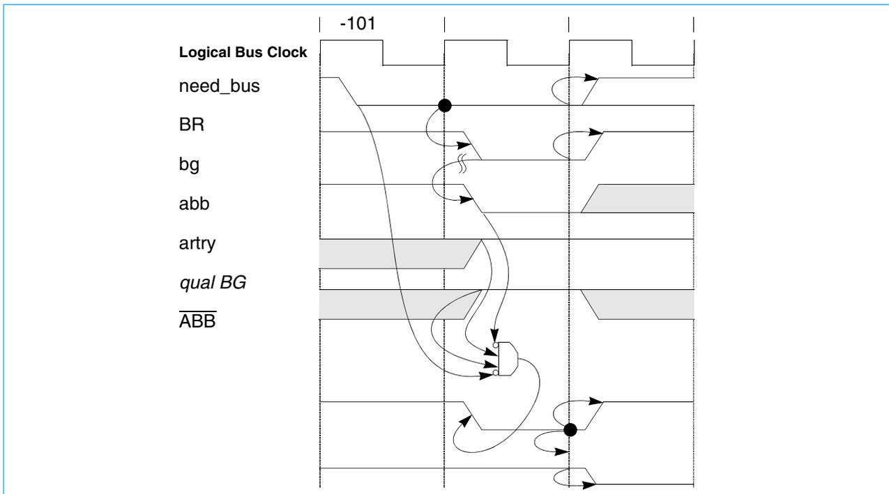
External arbiters must allow only one device at a time to be the address-bus master. For implementations in which no other device can be a master,  $\overline{BG}$  can be grounded (always asserted) to continually grant mastership of the address bus to the 750CL.
