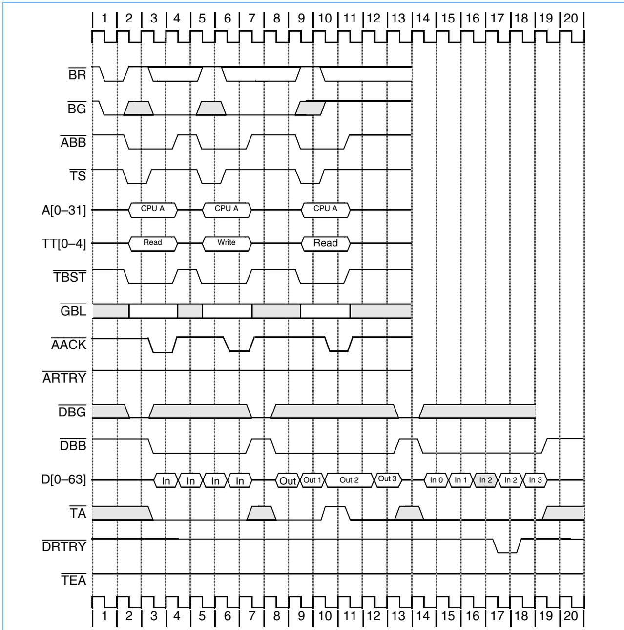
Figure 8-21 shows the use of the  $\overline{TEA}$  signal. Note that all bidirectional signals are three-stated between bus tenures. Note the following:
