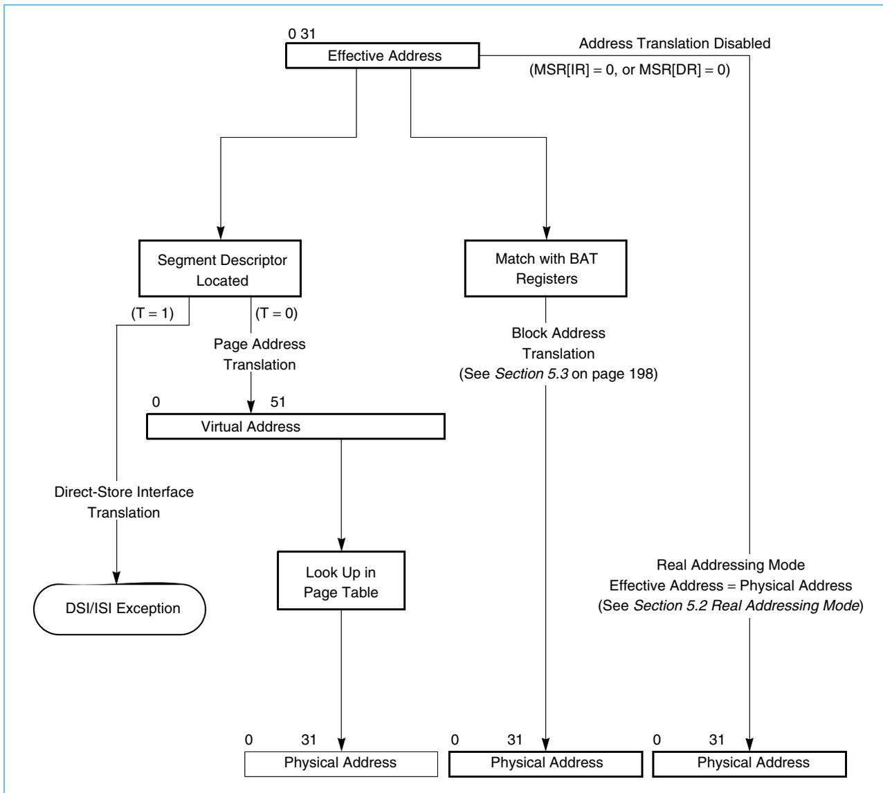
When the processor generates an access, and the corresponding address translation enable bit in MSR is cleared, the resulting physical address is identical to the effective address and all other translation mechanisms are ignored. Instruction address translation and data address translation are enabled by setting  $MSR[IR]$  and  $MSR[DR]$ , respectively.
