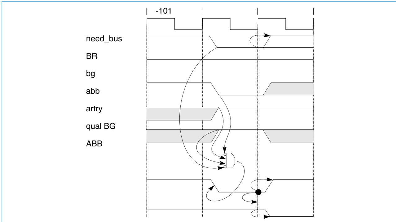
When the 750CL receives a qualified bus grant, it assumes address-bus mastership by asserting  $\overline{ABB}$  and negating the  $\overline{BR}$  output signal. Meanwhile, the 750CL drives the address for the requested access onto the address bus and asserts transfer start ( $\overline{TS}$ ) to indicate the start of a new transaction.
