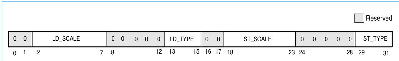
*Table 2-9* describes the bit fields for the GQR registers, and *Table 2-20* lists the encoding of the type fields in the GQR for the various quantized data types.
