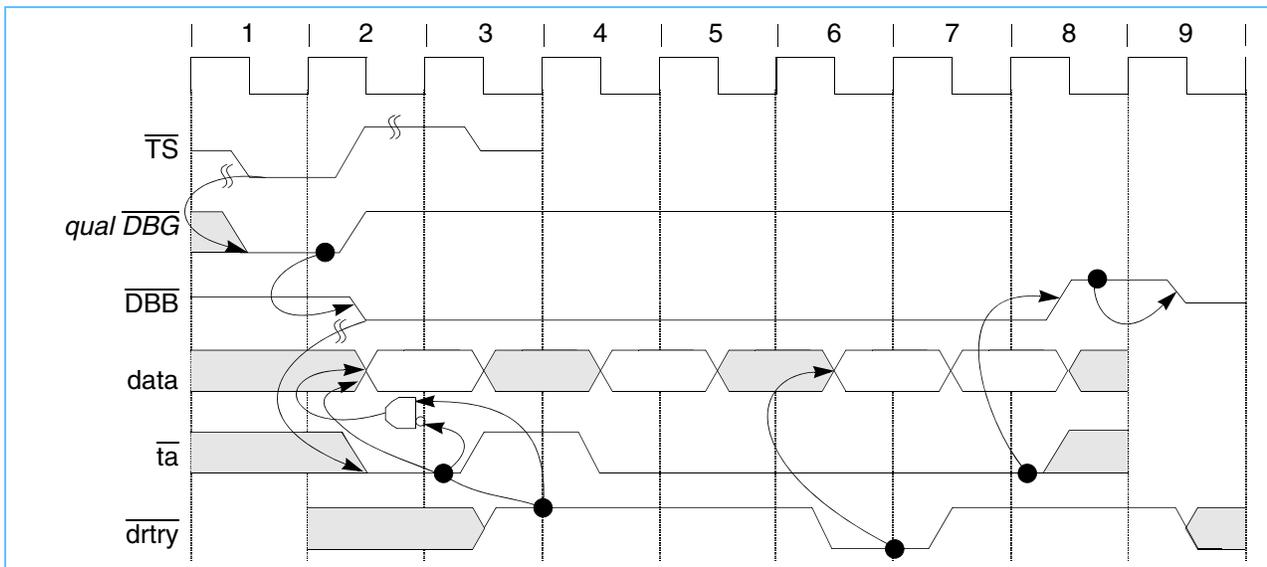
**Note:**  $\overline{DRTRY}$  is useful for systems that implement predicted forwarding of data such as those with direct-mapped, third-level caches where hit or miss is determined on the following bus clock cycle, or for parity-checked or ECC-checked memory systems. Also note that  $\overline{DRTRY}$  might not be implemented on other PowerPC® processors.
