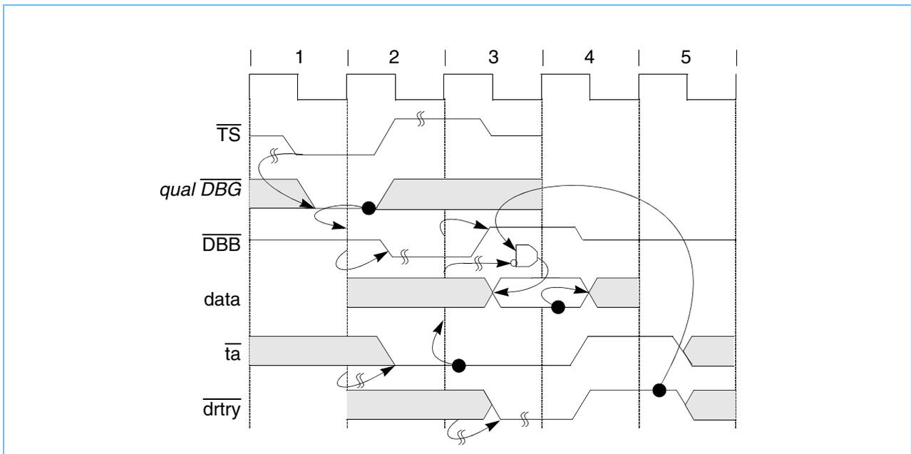
*Figure 8-14* shows the effect of using  $\overline{DRTRY}$  during a burst read. It also shows the effect of using  $\overline{TA}$  to pace the data-transfer rate. Notice that in bus clock cycle 3 of *Figure 8-14*,  $\overline{TA}$  is negated for the second data beat. The 750CL data pipeline does not proceed until bus clock cycle 4 when the  $\overline{TA}$  is reasserted.
