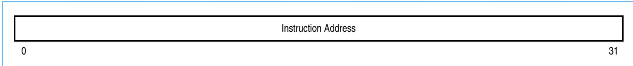
If the performance monitor interrupt is triggered by a threshold event, the SIA contains the exact instruction (called the sampled instruction) that caused the counter to overflow.
