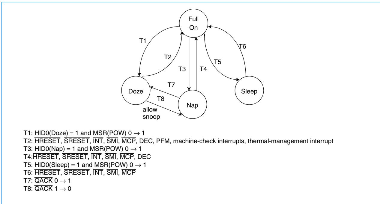
Hardware can enable a power management state through external asynchronous interrupts. Such a hardware interrupt causes the transfer of program flow to interrupt handler code that then invokes the appropriate power saving mode. The 750CL also contains a decremter which allows it to enter the nap or doze mode for a predetermined amount of time and then return to full power operation through a decremter interrupt.
