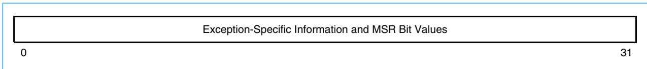
For most exceptions, bits 2–4 and 10–12 of SRR1 are loaded with exception-specific information and MSR[5–9, 16–31] are placed into the corresponding bit positions of SRR1.
