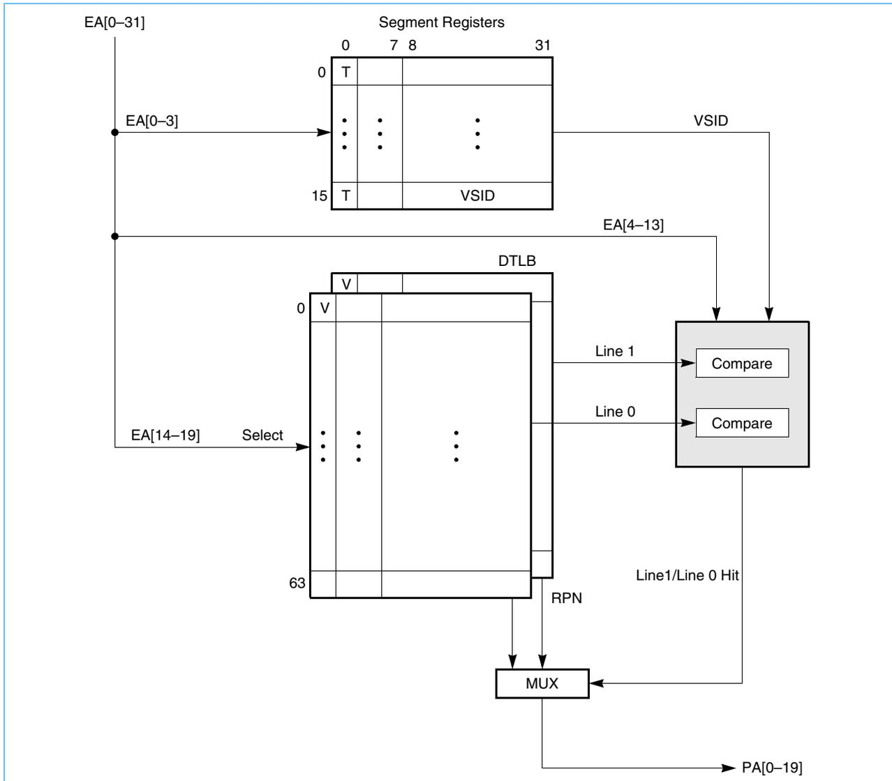
Unless the access is the result of an out-of-order access, a hardware table search operation begins if there is a TLB miss. If the access is out of order, the table search operation is postponed until the access is required, at which point the access is no longer out of order. When the matching PTE is found in memory, it is loaded into the TLB entry selected by the least-recently-used (LRU) replacement algorithm, and the translation process begins again, this time with a TLB hit.
