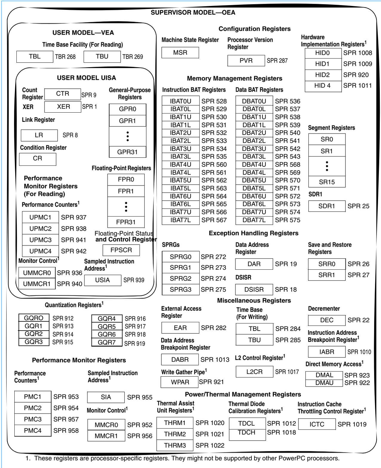
The PowerPC UISA registers are user-level. General-purpose registers (GPRs) and floating-point registers (FPRs) are accessed through instruction operands. Access to registers can be explicit (by using instructions for that purpose such as Move to Special-Purpose Register (**mtspr**) and Move from Special-Purpose Register (**mfspir**) instructions) or implicit as part of the execution of an instruction. Some registers are accessed both explicitly and implicitly.
