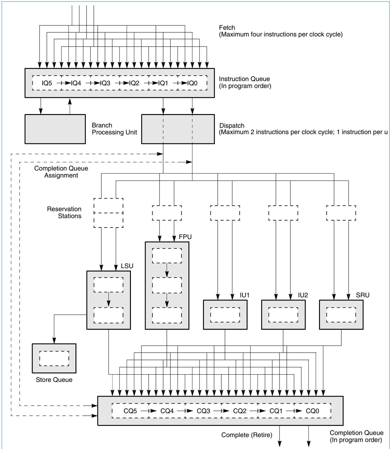
*Figure 6-5* shows a simple example of instruction fetching that hits in the L1 cache. This example uses a series of integer add and double-precision floating-point add instructions to show how the number of instructions to be fetched is determined, how program order is maintained by the instruction and completion queues, how instructions are dispatched and retired in pairs (maximum), and how the FPU, IU1, and IU2 pipelines function. The following instruction sequence is examined:
