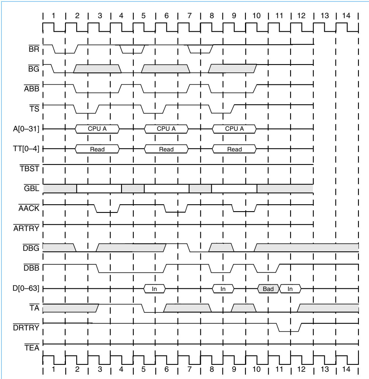
Figure 8-19 shows data-delay controls in a single-beat write operation. Note that all bidirectional signals are three-stated between bus tenures. Data transfers are delayed in the following ways:
