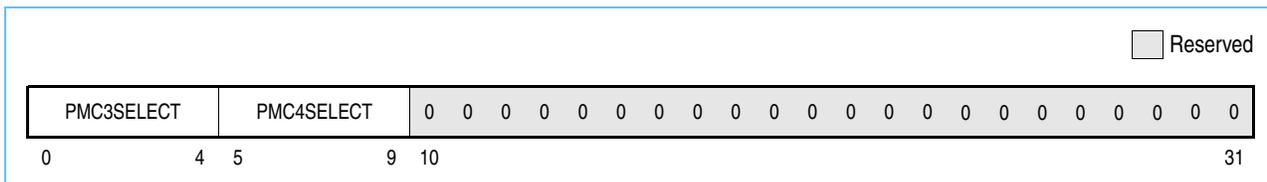
Bits for MMCR1 are shown in *Table 2-10*; the corresponding events are described in *Performance Monitor Counter Registers (PMC1–PMC4)*.
