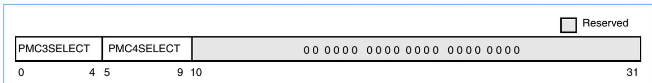
Bit settings for MMCR1 are shown in Table 11-3. The corresponding events are described in Section 11.2.1.5.
