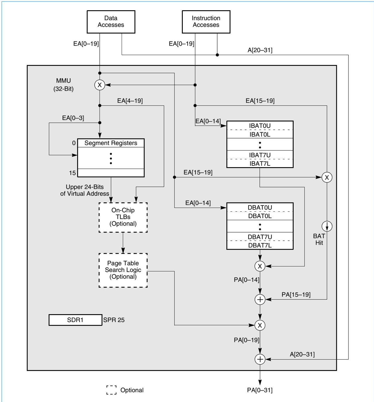
Figure 5-2. PowerPC 750CL Microprocessor IMMU Block Diagram
