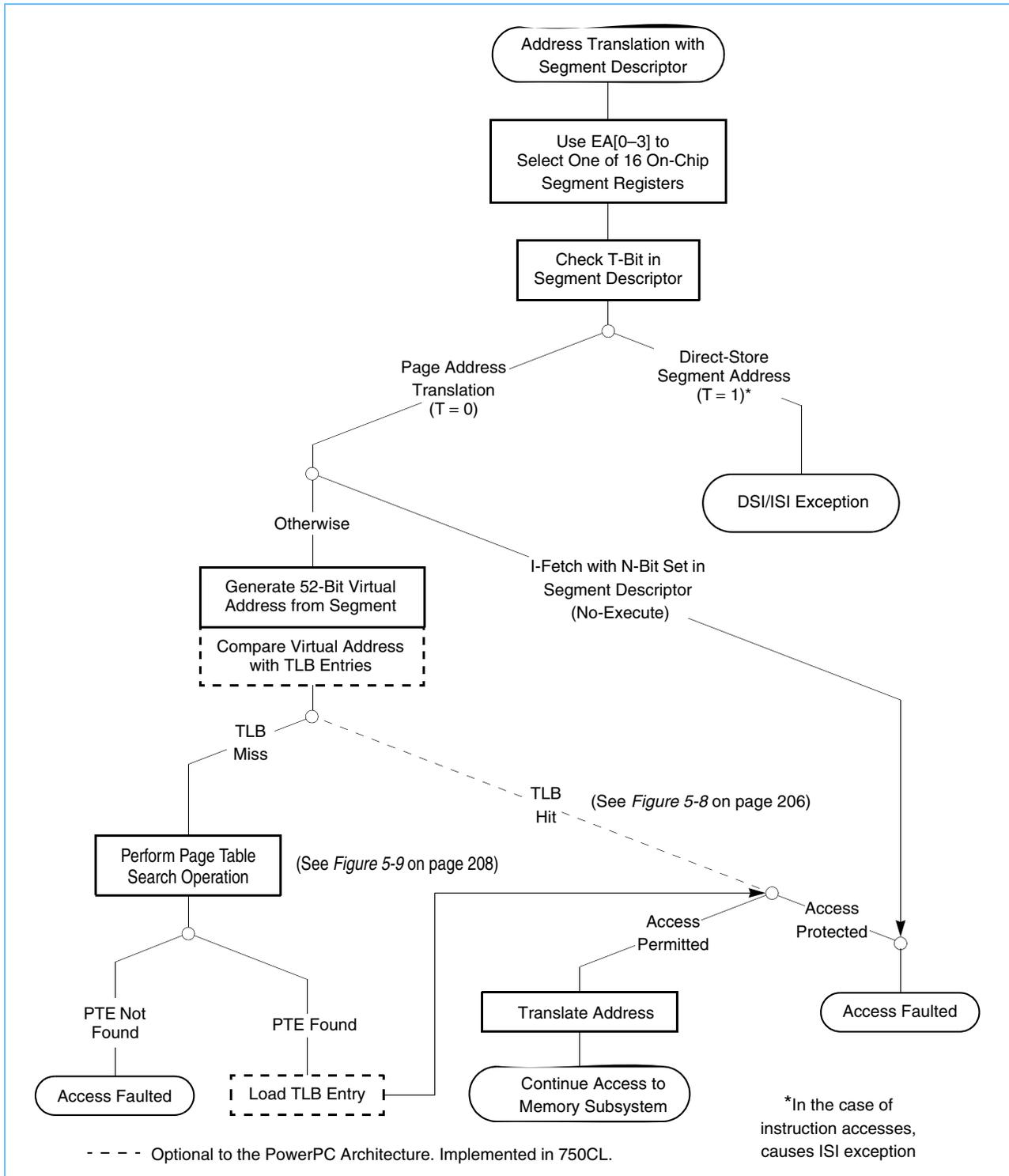
If  $SR[T] = 0$ , page address translation is selected. The information in the segment descriptor is then used to generate the 52-bit virtual address. The virtual address is then used to identify the page address translation information (stored as page table entries (PTEs) in a page table in memory). For increased performance, 750CL has two on-chip TLBs to cache recently-used translations on-chip.
