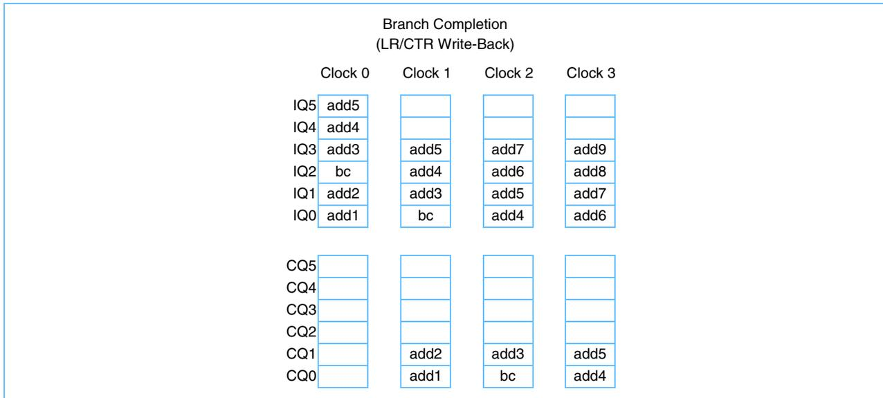
In this example, the **bc** instruction is encoded to decrement the CTR. It is predicted as not-taken in clock cycle 0. In clock cycle 2, **bc** and **add3** are both dispatched. In clock cycle 3, the architected CTR is updated and the **bc** instruction is retired from the completion queue.
