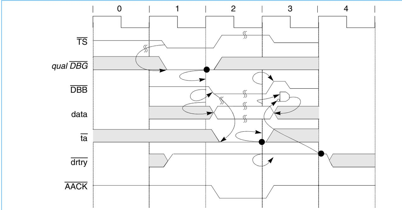
The  $\overline{DRTRY}$  signal is not sampled during data writes, as shown in *Figure 8-11*.
