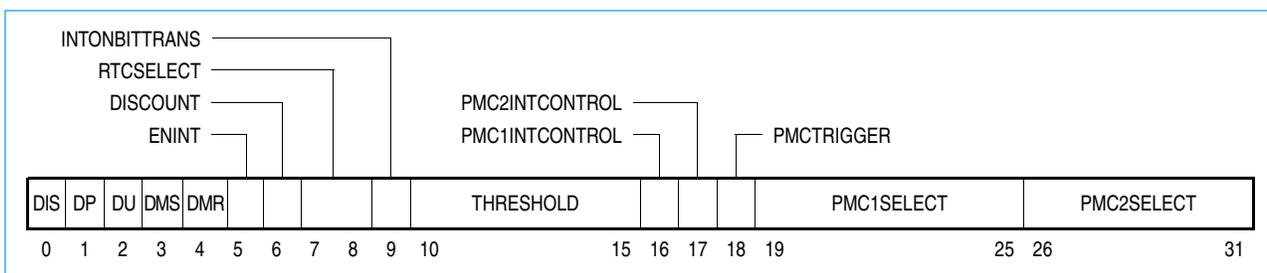
This register must be cleared at power up. Reading this register does not change its contents. The bits of the MMCR0 register are described in *Table 2-9*.
