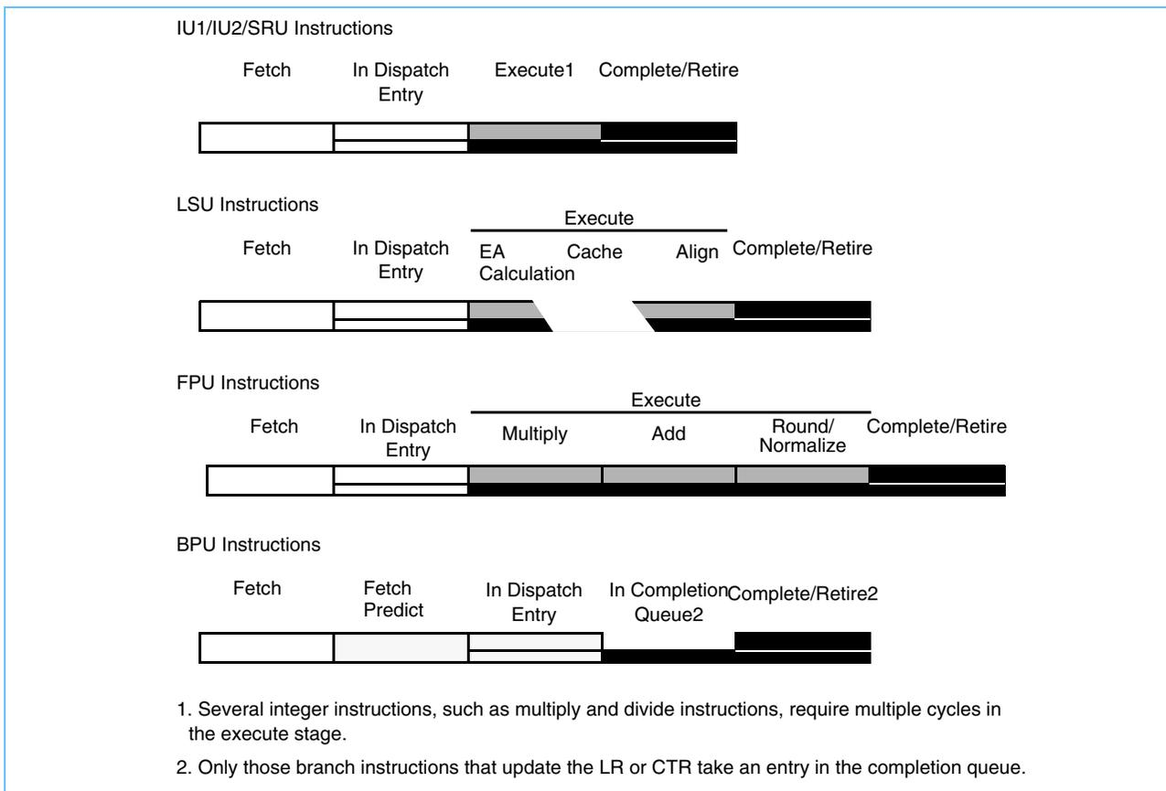
The 750CL's BPU decodes and executes branches immediately after they are fetched. When a conditional branch cannot be resolved due to a CR data (or any) dependency, the branch direction is predicted and execution continues on the predicted path. If the prediction is incorrect, the following steps are taken:
