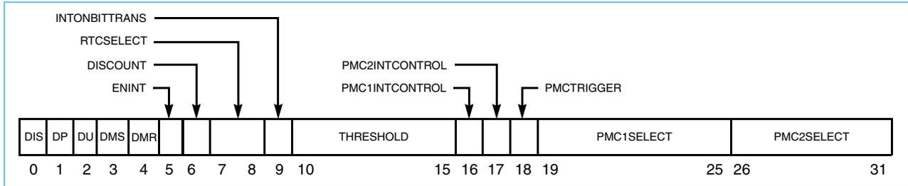
This register must be cleared at power up. Reading this register does not change its contents. *Table 11-2* describes the bits of the MMCR0 register.
