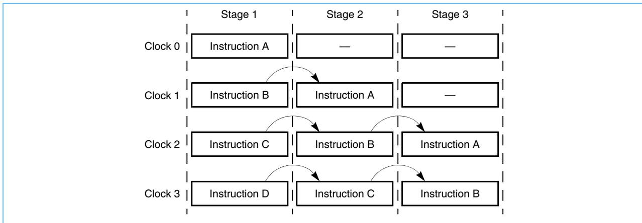
The 750CL can retire two instructions on every clock cycle. In general, the 750CL processes instructions in four stages—fetch, decode/dispatch, execute, and complete as shown in Figure 6-2. Note that the example of a pipelined execution unit in Figure 6-1 is similar to the three-stage FPU pipeline in Figure 6-2.
