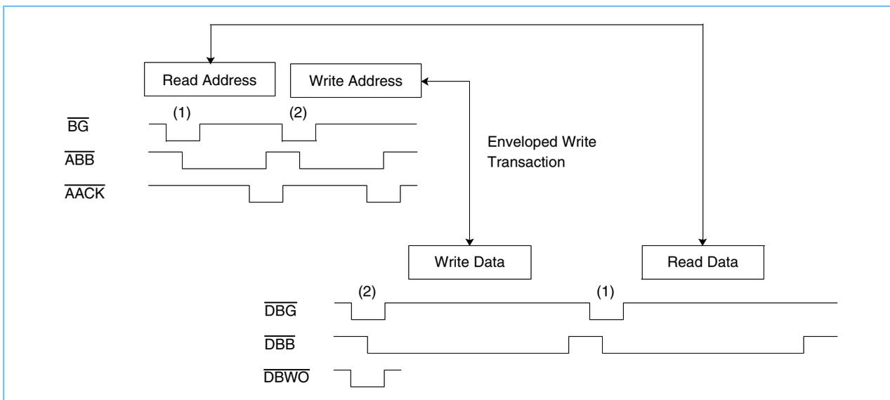
Note that although the 750CL can pipeline any write transaction behind the read transaction, special care should be used when using the enveloped write feature. It is envisioned that most system implementations will not need this capability; for these applications,  $\overline{DBWO}$  should remain negated. In systems where this capability is needed,  $\overline{DBWO}$  should be asserted under the following scenario:
