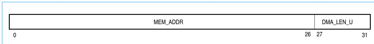
Figure 2-17. Direct Memory Access Lower (DMAL) register
